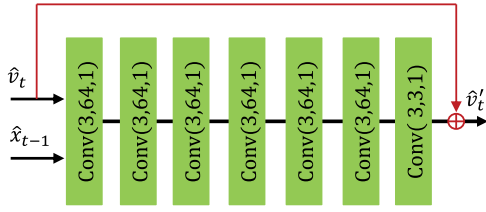
Fig. 8. The network architecture of our motion refinement network.
